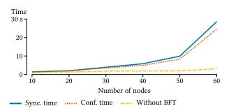
**Figure 4.** Increasing synchronization and confirmation times for different number of nodes for the 99th percentile.
